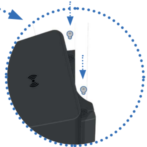
09 Tightening the head two bolts from above
