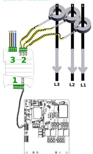
According to the above diagram for proper operation, three plugs connection is required (3-phase configuration):
