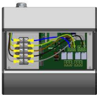
Fig. 23: Electrical connection executed correctly.
