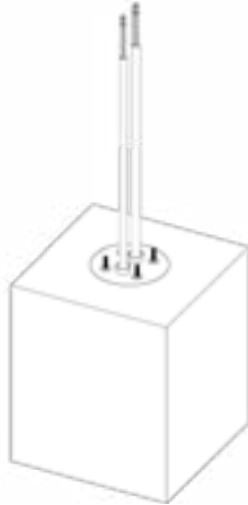
Fig. 22: Properly constructed foundation using the prefabricated element.
