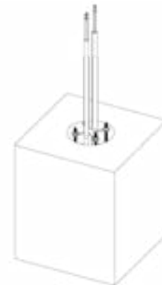
Fig. 29: Foundation set correctly placed in the excavation
