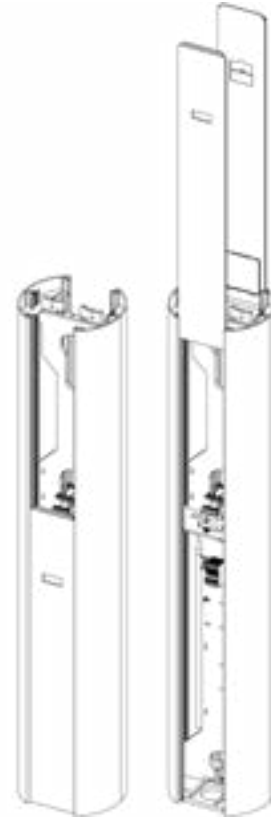
Fig. 34: Sliding the lower masking panels out of the ENELION VERTICA Pole.
