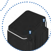
09b Tighten the head – two long bolts at the bottom and two screws at the top
