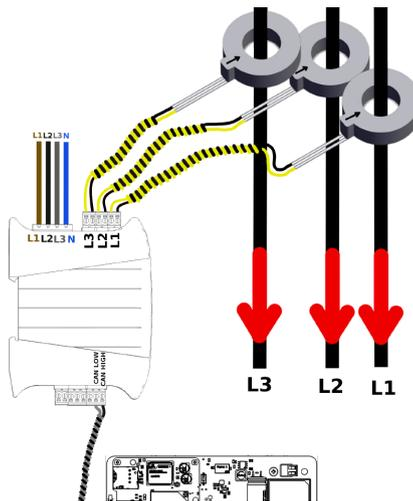
**Fig. 5:** Connection diagram for the 3-phase variant of ENELION ENERGY GUARD.
