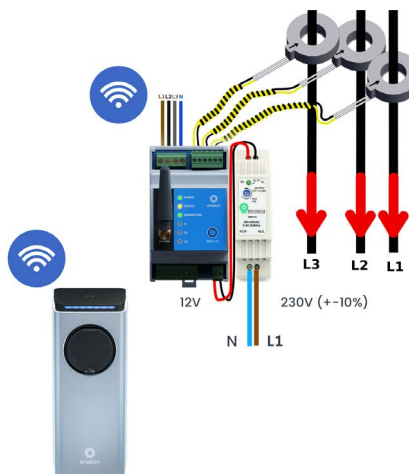
Fig. 5: Connection diagram for the 3-phase variant of ENELION ENERGY GUARD.
