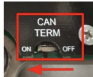
Fig. 63: CAN bus termination switch on the Enelion-VERTICA link module. To enable termination, set the switch to the "ON" position.
