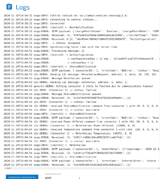
fig. 22: Logs section of the System tab.
