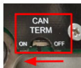
Fig. 52: CAN bus termination switch on the Vertica link module. To enable termination, set the switch to the "ON" position.
