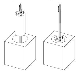
Fig. 16: Placing the prefabricated element in the excavation.
