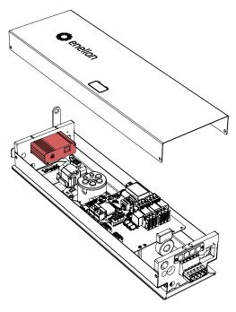
Fig. 62: Mounting the LTE module.
