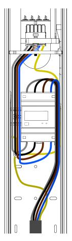
Fig. 38: Example of Vertica Pole connection with the use of MID meter.
