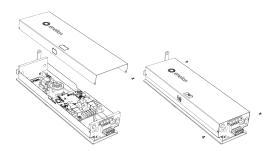
Fig. 60: Closing the Vertica Module with RCM B.
