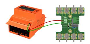
Fig. 39: MID meter connection diagram.
