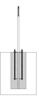
Fig. 25: Cross-section of the foundation set cast in the concrete
