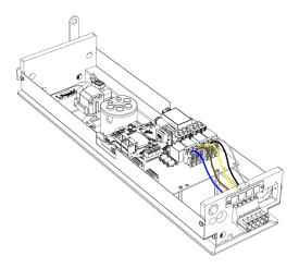
Fig. 57: The charging controller power connector on the Vertica Module.
