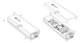
Fig. 52: Opening the Vertica Module.
