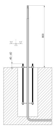
Fig. 22: Diagram of placing the foundation set in the excavation
