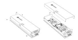
Fig. 61: Mounting the LTE module.
