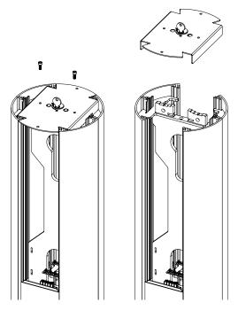
Fig. 6: Removing the lock plate.
