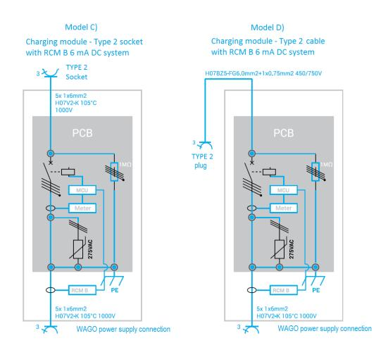
Fig. 13: Pictorial diagrams of Vertica Modules part 2/2.
