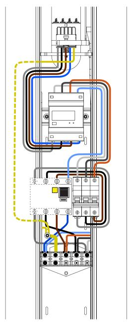
Fig. 49: Obverse of the Vertica Pole after mounting the Vertica Splitter with the MID meter present.
