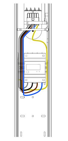
Fig. 35: MID meter fitted in Vertica Pole.
