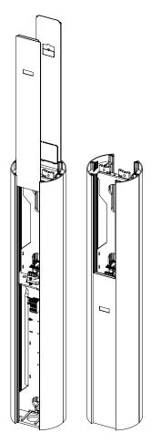
Fig. 51: Inserting the lower masking panels into Vertica Pole.
