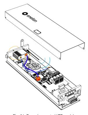
Fig. 64: Properly mounted LTE module.
