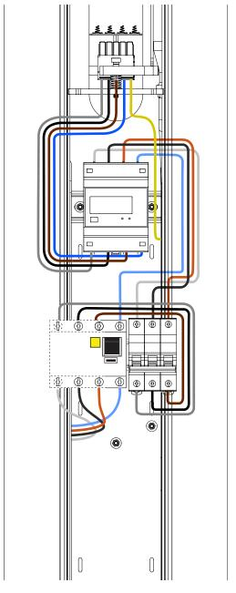
Fig. 50: Reverse of the Vertica Pole after mounting the Vertica Splitter with the MID meter present.
