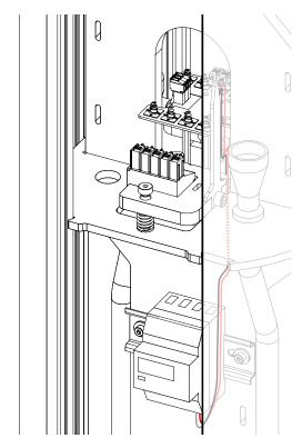
Fig. 36: Routing the MID meter signal cables.
