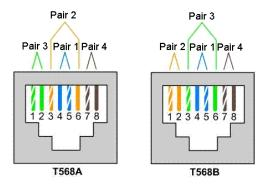
Fig. 45: Ending the Ethernet Patchcord according to TIA-568A/B do 100BaseT
