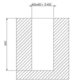
Fig. 15: Diagram of the foundation excavation.
