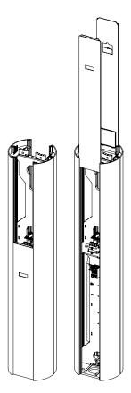
Fig. 28: Sliding the lower masking panels out of the Vertica Pole.
