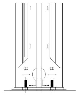
Fig. 31: Mounted and bolted Vertica Pole.
