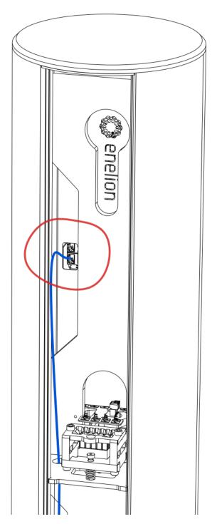
Fig. 48: Cable routed to the Ethernet socket.
