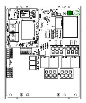
Fig. 63: Location of the power socket for LTE module power cable
