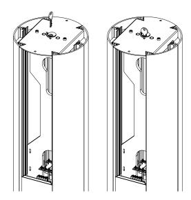
Fig. 5: Unlocking the lock plate.
