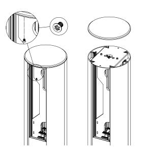
Fig. 4: Removing the cover of the Vertica Pole.
